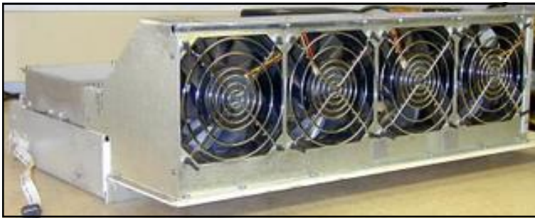
Completed Air Plenum
