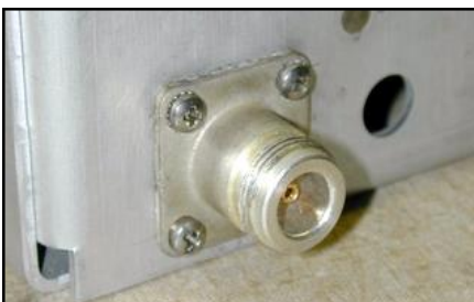
New RF output connector on chassis
