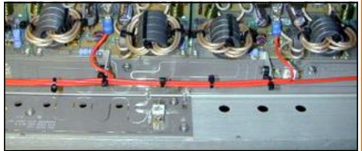
1/4 Module Component Cooling Holes
