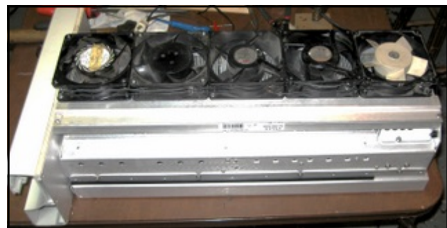
Impingement / Jet Cooling
