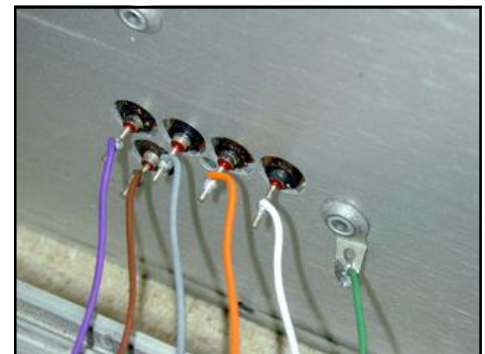
Front Panel LED Blink Code Wires
